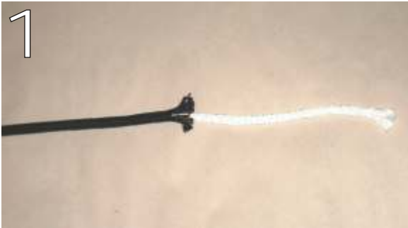
Slide the cover back to expose about 1 foot (300mm) of core.
