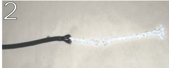
Cut off about 8" of core and taper about 3" of the end of the core. This allows the core to be put inside the cover so it is easier to pull into the throat of the eye.
