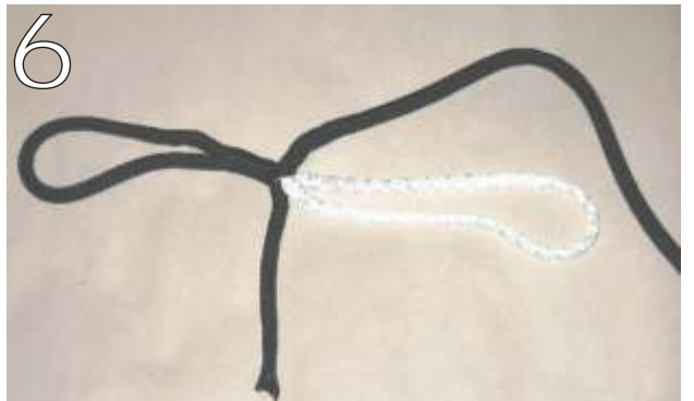
Right where the cover comes out bend the rope sharply and extract the core making a loop of it as shown below. This will take some digging but it can be done without too much difficulty. The end result is shown in this photo.
