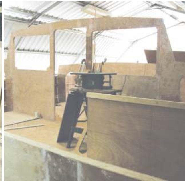
The pine frames faced with marine ply
