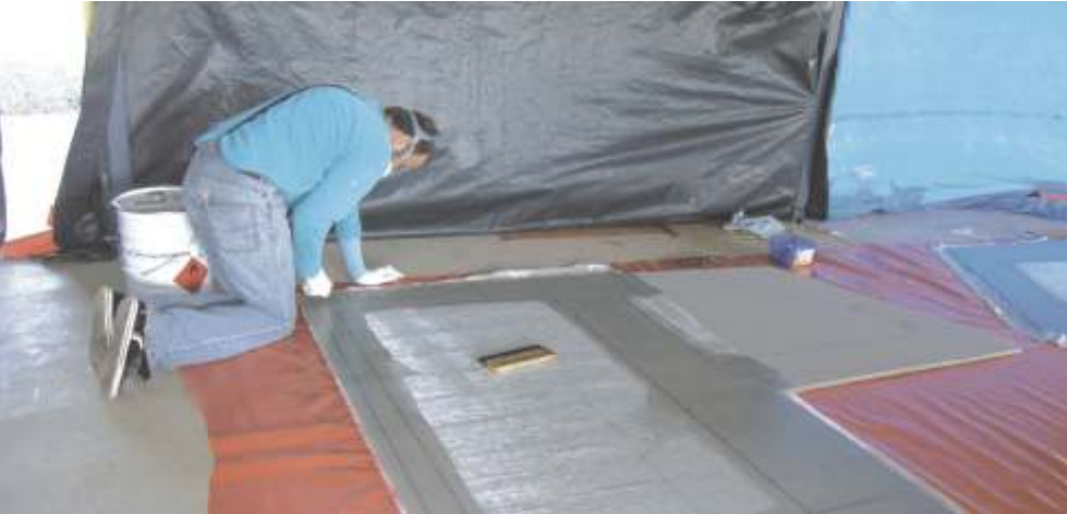
This is the last project done before this printing. I am laminating 15mm foam that I have marked for apertures to be cut out later. I did this bulkhead in halves and joined later.
