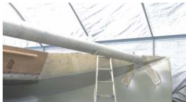
With the forebeam in place the decks can be installed, another important milestone.
