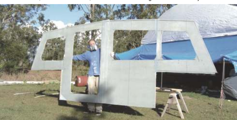
The "finished" product is light, strong and relatively inexpensive (I won't use cheap though). I left some material around the edges for final shaping. I also left the protective "peel ply" covering in place for now. NOTE THE SAFETY GEAR! ALWAYS!
