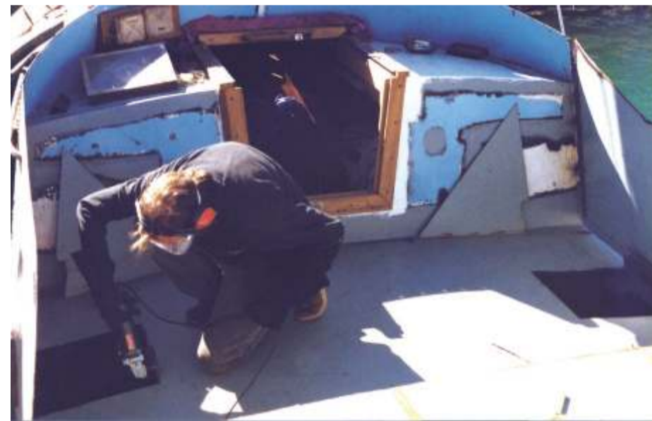
This centre cockpit design was unusual in that instead of an engine under the cockpit, that was our galley. This was OK in that we had a beaut of a galley but it suffered from lack of light and ventilation. The triangular shaped boxes reflected a good amount of light and they ventilated from a sheltered position. A very successful addition.
