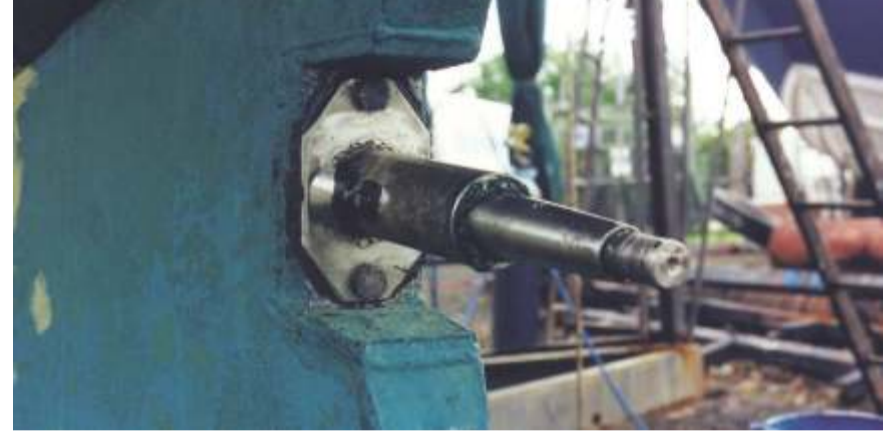
Reconstructing the stern tube and cutlass at the slip way, all from 316 stainless
