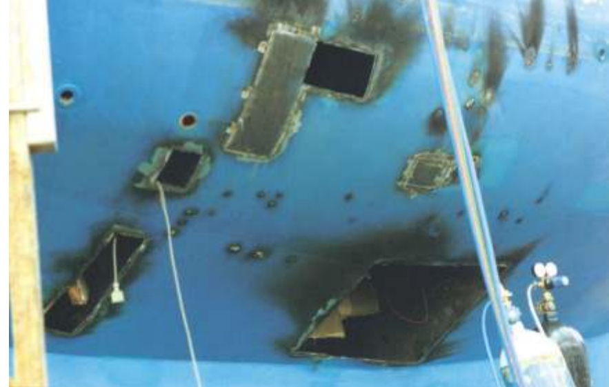
Reconstructing the stern tube and cutlass at the slip way, all from 316 stainless
