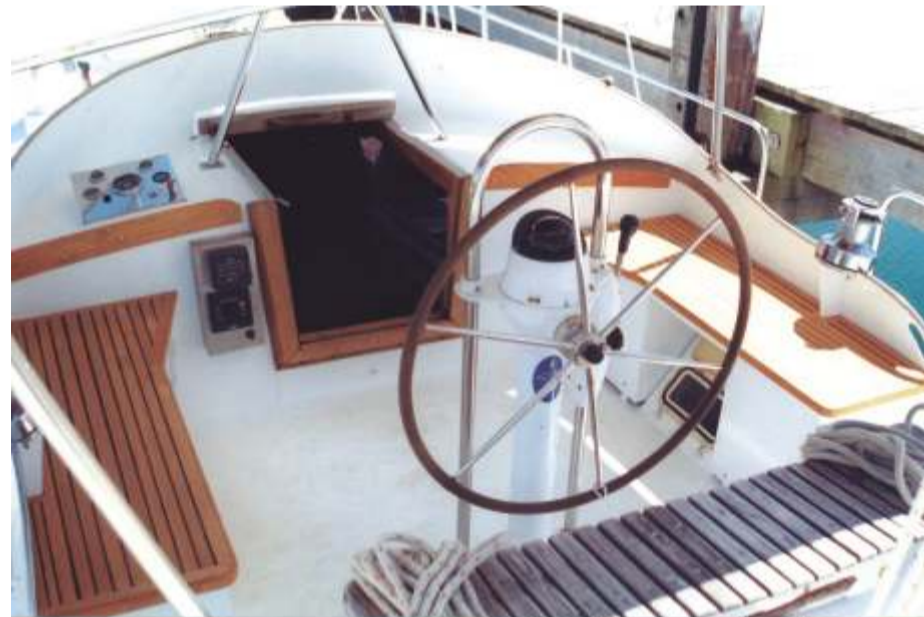
Teak is so attractive against a white surface. The little that was used was screwed in place to allow occasional service. The lockers were ply suspended above the deck by steel tabs. It was all set up to flow water through full length scuppers under the combing. The hard dodger and combing are edged in 5/8" stainless tube.
