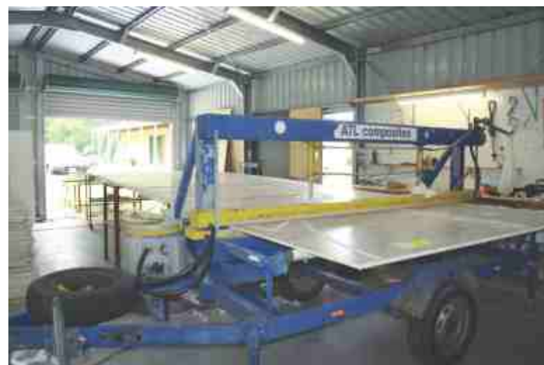
The first step in the process is gluing the panels together Then cutting the pre-routed shapes out.
