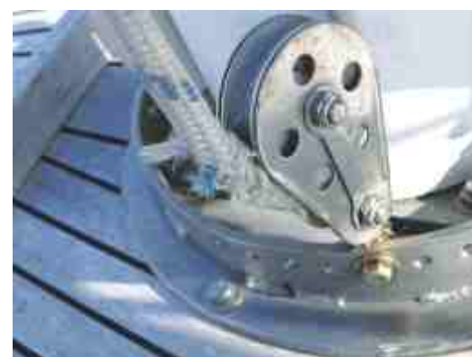
Above: an example of halyard chafe. To right: If you must cover the rigging wire make sure the lower end of the cover doesn't trap moisture and debris.
