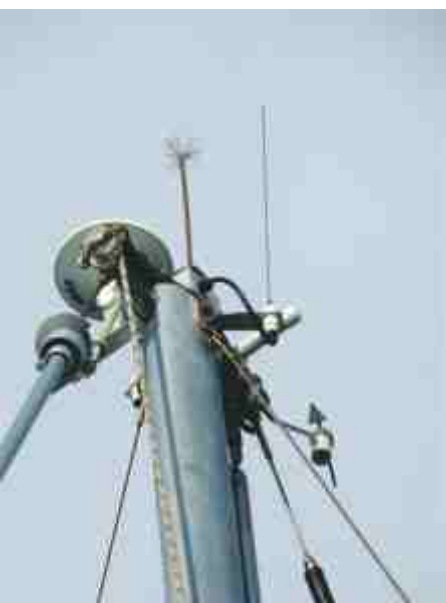
Above: How to trap salt-laden moisture and dirt, promote corrosion and make your sails nice and dirty too!
