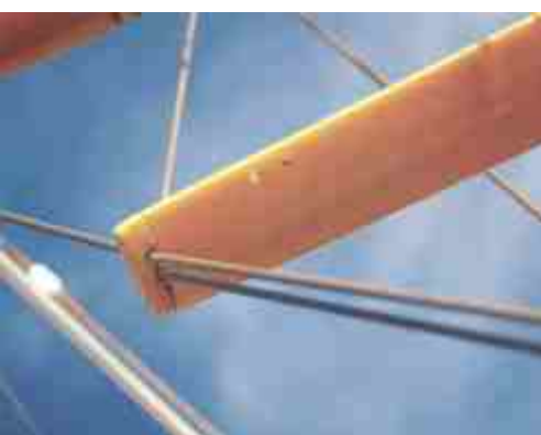
Neat spreader-end clamp. Be sure to coat the aluminium with Duralac to discourage corrosion between dissimilar metals.
