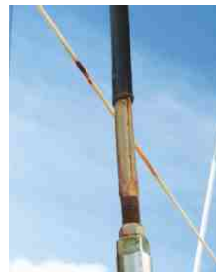
Above: an example of halyard chafe. To right: If you must cover the rigging wire make sure the lower end of the cover doesn't trap moisture and debris.
