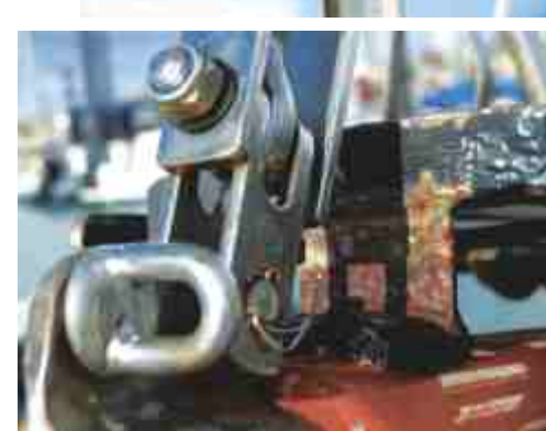
How not to use a split pin! And the clevis pin is undersize for the hole in the toggle.
